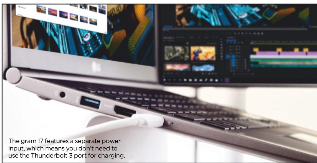
The gram 17 features a separate power input, which means you don't need to use the Thunderbolt 3 port for charging.
