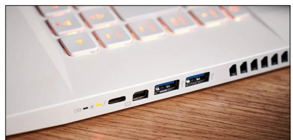
There are ports a-plenty on the Acer ConceptD 7, including USB-A and USB-C, and an Ethernet port. Note: the series of oddly shaped holes are just vents!
